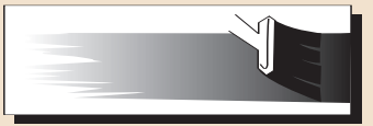
Feathering Technique, use only if stopping in the middle of a log is unavoidable.
